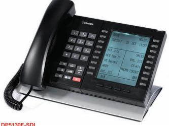
Digital hands-free featurephone with 10 programmable keys and a large 9-line, backlit, LCD display for full on-screen prompts.
